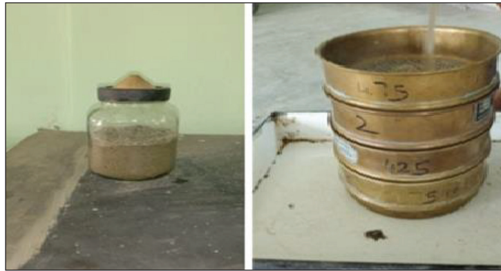
Figure 1. The specific gravity of PA and grain size analysis of pond ash
